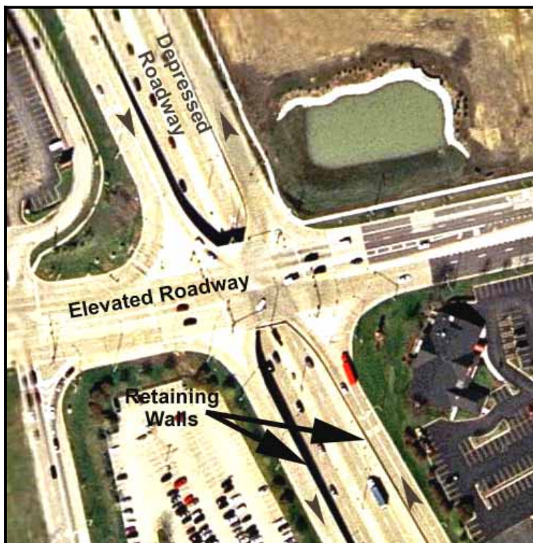
Figure 3 Single Point Diamond Interchange Illustration
